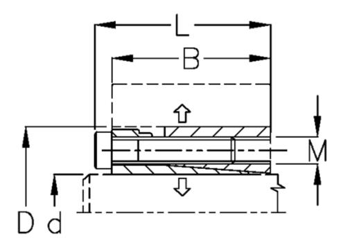
B mm = 76d H8 mm = 140D mm = 190Fit tolerance = Aksel h8, Nav H8
